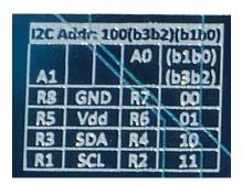
Resistors R1-R8 are used to select the I<sup>2</sup>C slave address.
